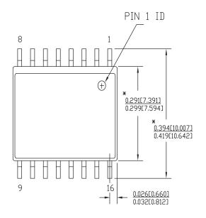
DIMENSIONS IN INCHES[MM]  $\frac{\text{MIN.}}{\text{MAX.}}$  REFERENCE JEDEC MO-119
